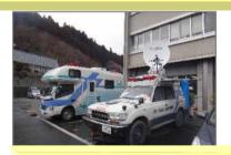
Satellite communications vehicle used to secure disrupted communication lines
