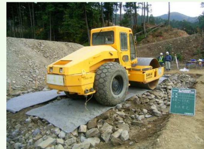
Rupture test of waterproof sheet
