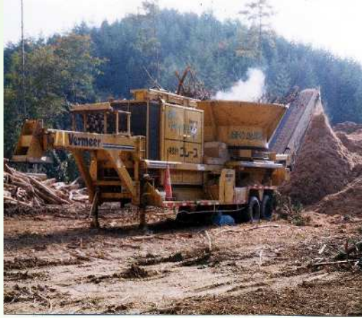
Trees are chipped using a tab grinder
