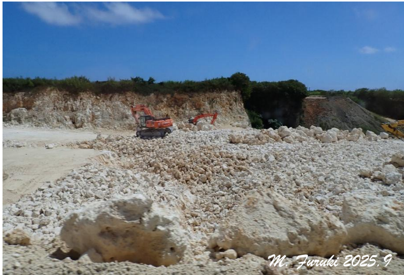
Quarry, quarrying is possible with a ripper without using blasting
