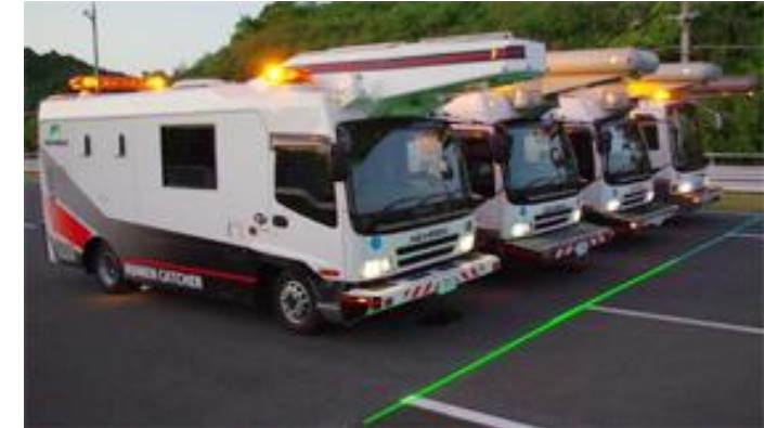
Road surface survey car (Nichireki)
