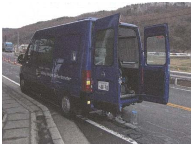
Photograph-3.2.1: Measurement of asphalt pavement surface with FWD
