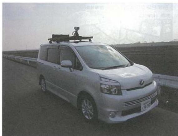
Appendix Photograph-3.4.1: Automatic road surface photographing vehicle
