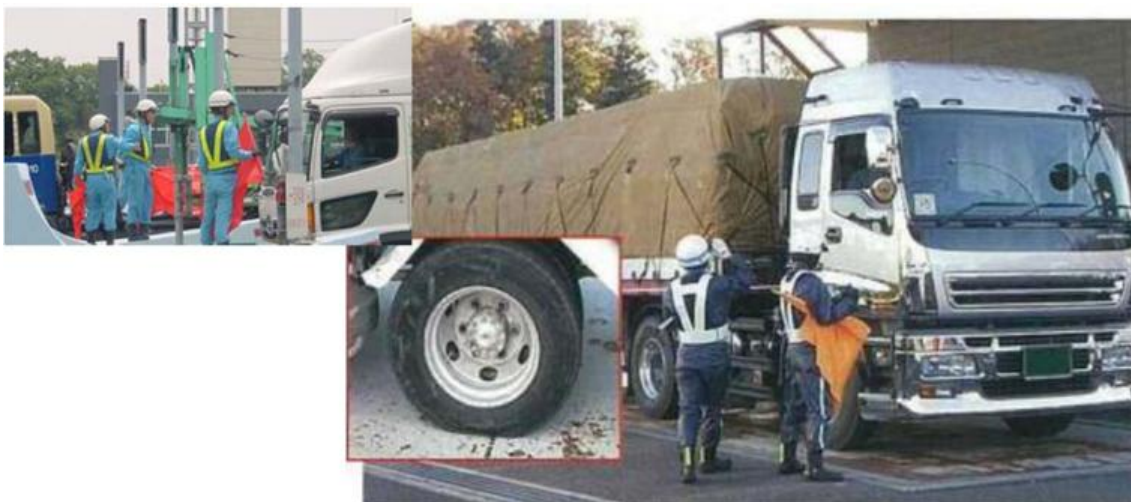
Appendix Photograph-9.4.3: Measurement of total weight after guiding a vehicle from a toll booth to a measurement area 5)
