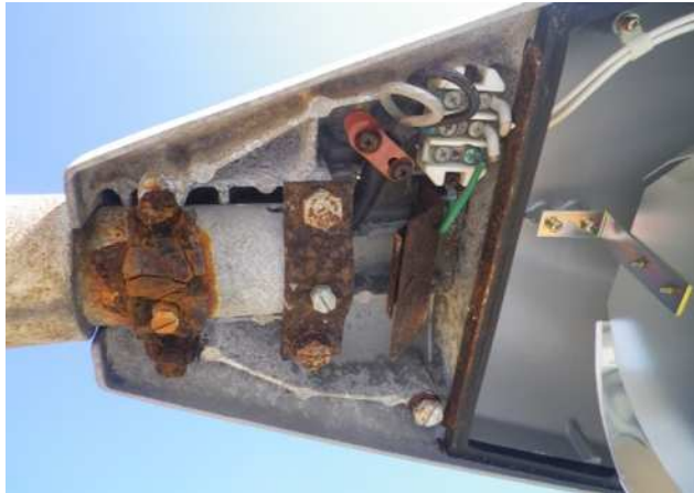
Corrosion due to dissimilar metal contact at the lamp mounting area
