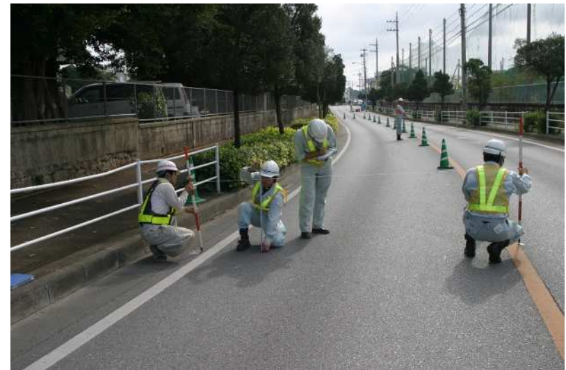
Measurement of rutting depth
