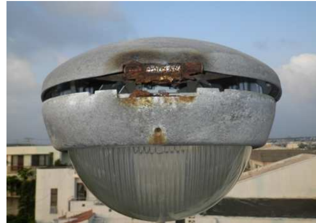
Breakage due to dissimilar metal contact corrosion at the opening of the lamp
