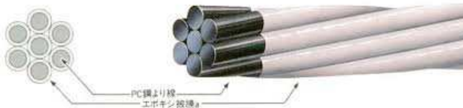
All-strand epoxy resin coated PC steel strand
