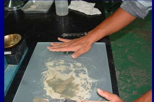
Plasticity limit test status
