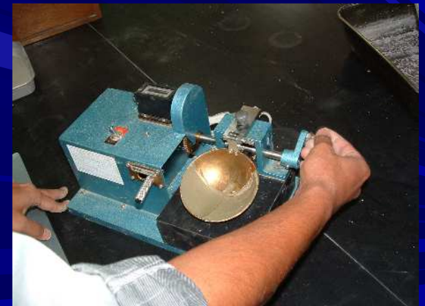
Liquid limit test status
